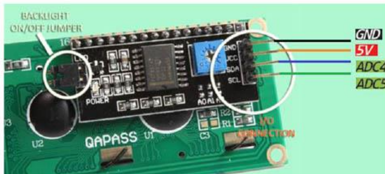
LCD display to Arduino wiring.
